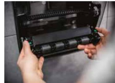
Fully opening cutting mechanisms.
